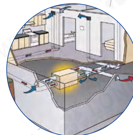
Primary Air System
